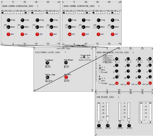
Figure 3. Interconnected Datatonism modules, with Pure Data patch cables replacing the hardware connections at top and bottom only.
