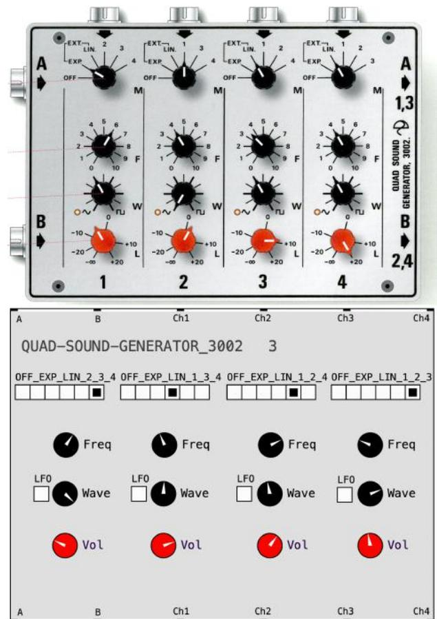
Figure 2. Comparison of the original analog (top) [3] and digital emulation (bottom) versions of the Quad Sound Generator module.
