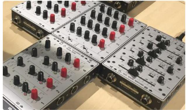
Figure 1. Interconnected Dataton modules. Note the hardware connections on all four sides of each module.
